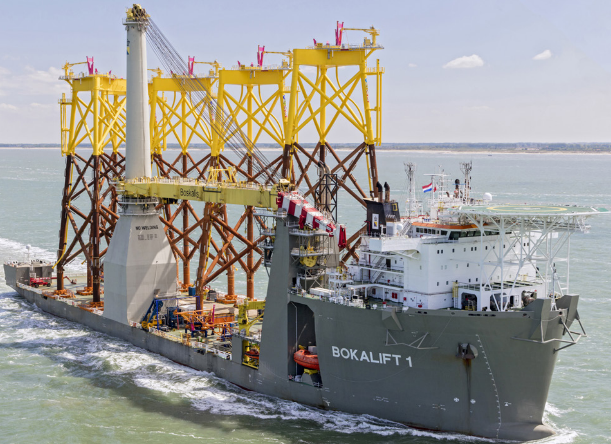
The Bokalift 1 demonstrating its unique capabilities by transporting and installing five giant jacket foundations in one go for the East Anglia wind farm
