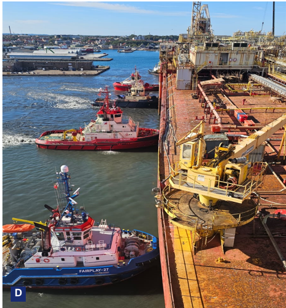
D FPSO berthing operation in Frederikshavn, Denmark using harbour tugs
