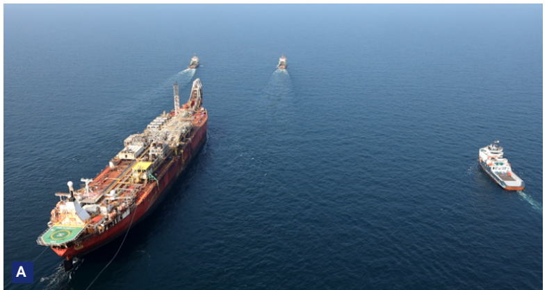
A FPSO tow with two leading ocean tugs and one escort tug. Also note trailing on the back of the FPSO the messenger lines for the two emergency towing lines hanging on the FPSO side that can be deployed without any assistance from the unmanned FPSO
