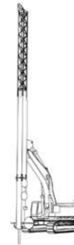
Cofra developed the BeauDrain-S system in order to be able to apply vacuum drainage to surfaces and installation depths of any size. BeauDrain-S combines the standard BeauDrain system and vertical drainage. With this technique, sand layers are blinded off by a polythene hose and the drain is applied only in the compactable layer. This technique can be applied in specific soils anywhere in the world, on any surface and at any depth.
