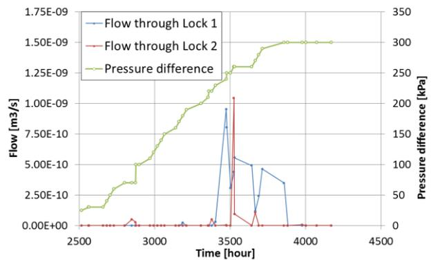
Fig. 3. Flow through 1.25m long lock sections in time with increasing pressures.
