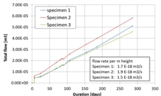
Fig. 4. Long term measurements of the water flow through three 1.25m long lock sections after complete seal.
