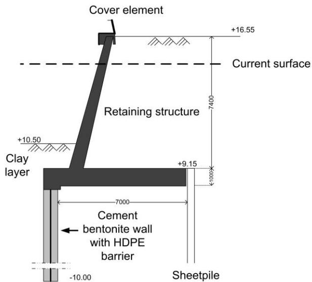
Fig. 11. Structure of the retaining wall (after Effing, 2014).
