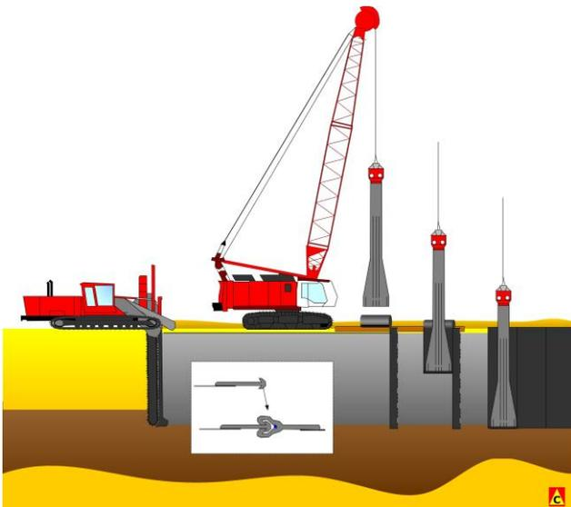
Fig. 5. Installation procedure of the barrier using a trencher.
