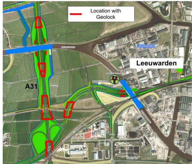
Fig. 6. Location of the HDPE barriers (modified from <http://www.vrij-baan.nl>).
